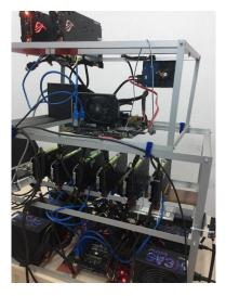
**Figure 3** – Example of cryptocurrency miner setup: at the bottom level Setup #1 is shown; at top Setup #2 is shown. We compare data to the average power consumption of Desktop PC with LCD Display [15].
