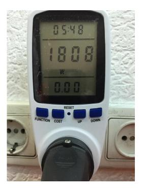
**Figure 2** – Power Meter Energy Monitor TS-836A shows the power consumption of setup #1 consuming an average of 1,800 Watts per hour running on the sample rate of 5 minutes.
